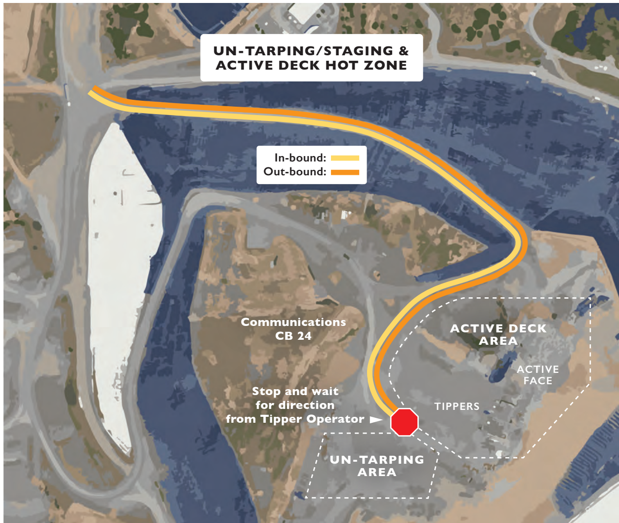
Figure 3. Un-Tarpping/Staging and Active Deck Areas
