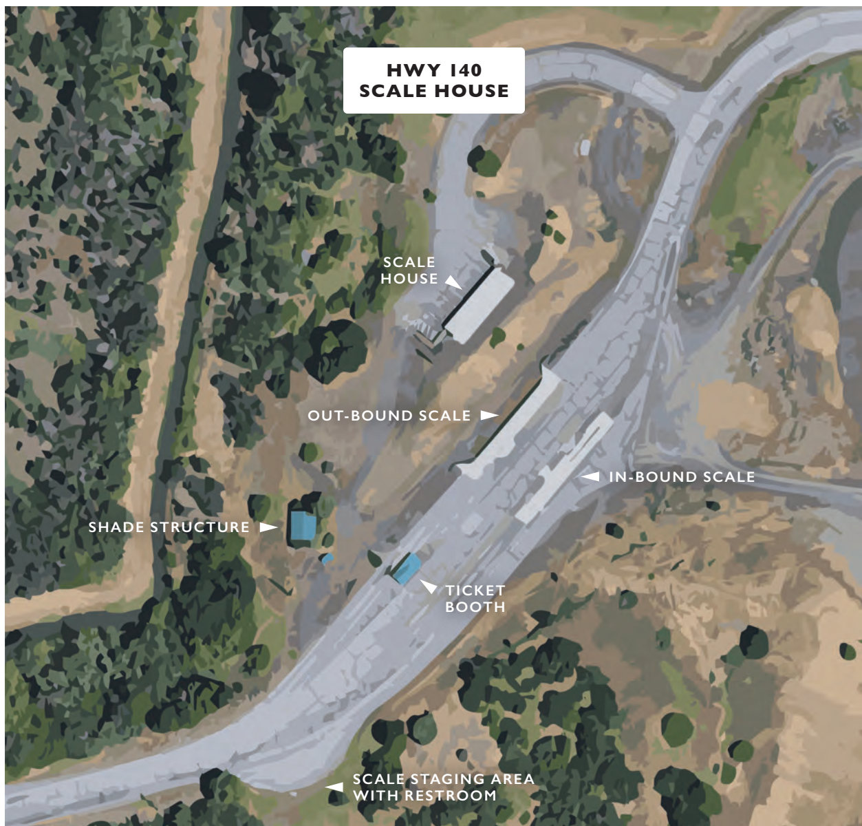
Figure 1. HWY 140 Scale House
